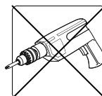
We do not recommend the use of power drill/drivers for inserting screws, as this could
