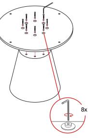
attach the connecting board to the table base "
