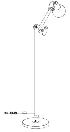
**Caution**: If the external flexible cable or cord of this luminaire is damaged, it should be replaced by a qualified person in order to avoid a hazard.
