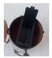
3. Insert two AA batteries properly as the mark on the battery case.
