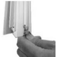
Fasten the profiles together by sliding the square headed bolts into the channel of the profile and attach to the hole in the corresponding bar. Do not tighten the nuts completely until the completed frame is square. **NOTE THAT ALL CONNECTING PROFILES MUST BE FLUSH AND TIGHT TOGETHER TO ENSURE THAT LEAKING IS KEPT TO A MINIMUM.**
